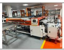
**EVA Cutting Machine** - Auto feeding EVA coiled material, auto cutting and punching, and laying it on the glass.
