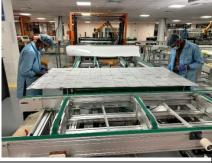
**Bussing** - After arranging strings, connect them to each other with a busbar (soldering).
