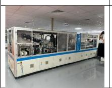
**Stringer-** Soldering equipment for serial connection between cells, Compatible with 5BB-9BB, 156-158.75 mm cells.
